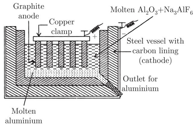
Electrolytic cell for the extraction of aluminium
